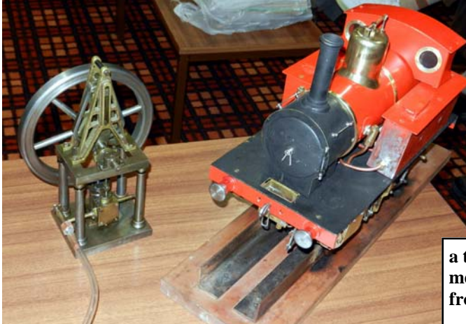
a "Table Engine" a together with a rebuilt "Tich" 3 1/2" gauge locomotive by Russell Gifford.
